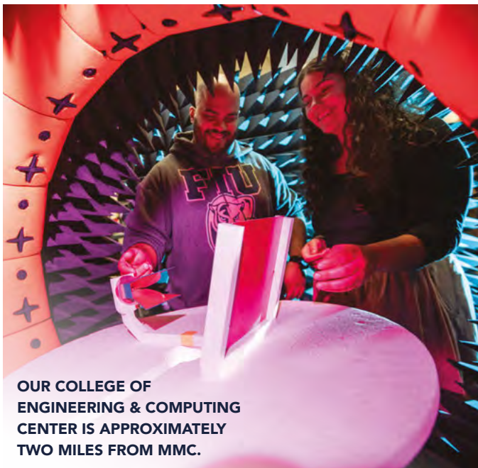
Ph.D. student Carlos Velez and undergraduate student researcher Briana Gonzalez measure an origami reflectarray antenna for CubeSat applications at the Transforming Antennas Center, which is directed by Professor Stavros Georgakopoulos.
